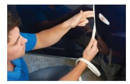
For a fixed part, like the A Post, apply to the panel edge making sure the adhesive is behind the panel. Press evenly and firmly for good adhesion.
