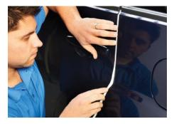
Close the moving part very carefully and then do a visual check to make sure there is no exposed adhesive.
