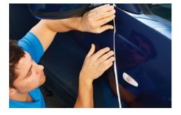
Close the part carefully to make sure the foam is exposed then smooth the tape into the gap with your finger to the required depth.
