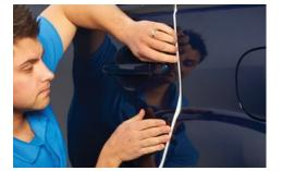
Close the part and smooth the foam tape into the gap with your finger to the required depth.
